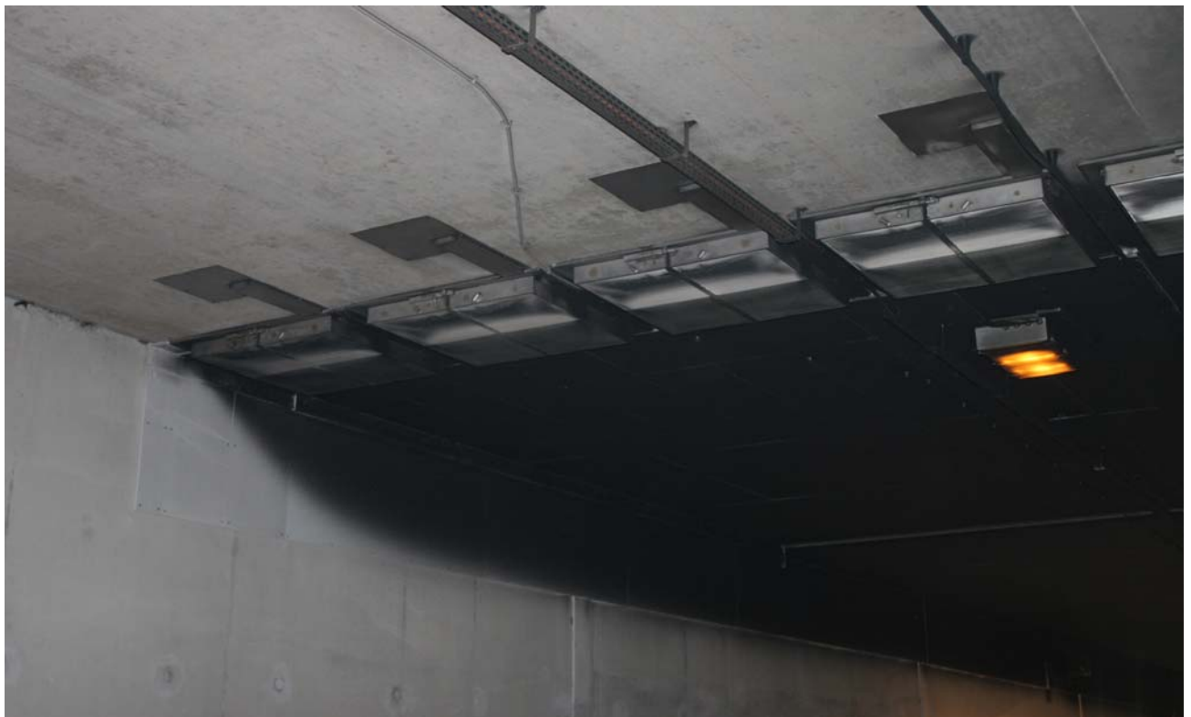
Picture 57: After the test, there was a blackened 1 m high strip to be seen on the southern wall next to the ceiling, extending over 100 m from the smoke extracting station #05 to the next one. The accurate border line of the black soot gave proof of the precise flow of the smoke layer during the entire test. The same traces from the stratification could be seen at the smoke extracting station #06 after the test.
