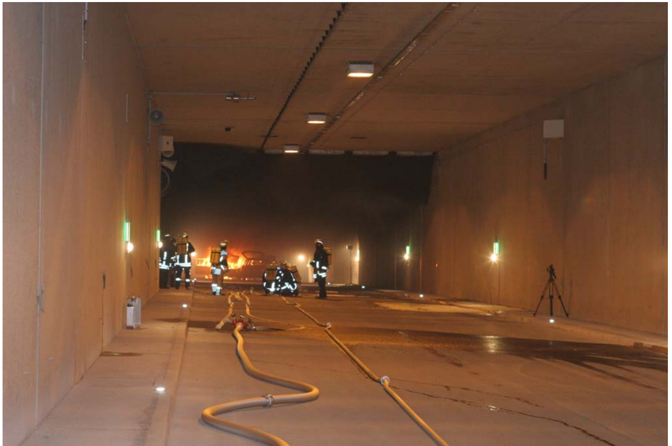
Picture 31: The burning of two cars after the flash-over of the fire, viewed after 25 minutes from the east, the flow of the smoke layer was still stable when moving towards the smoke extracting station #6, all safety apparatus can be seen on the wall (the encapsulated ultra-sonic meter and the loud speakers) or below the ceiling (the ECS, the opacimeter, the black radio antenna and the white heat sensor cable).
