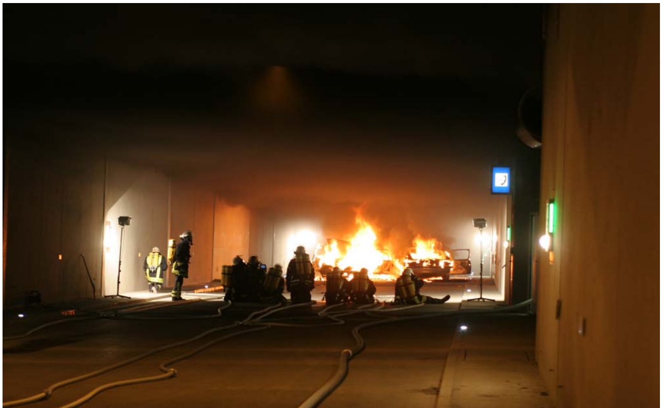
Picture 42: There was a maximum HRR of 12 MW from the burning cars, viewed after 24 minutes from the west, and still there was a stable smoke layer as the fire brigade organised for the near attack.
