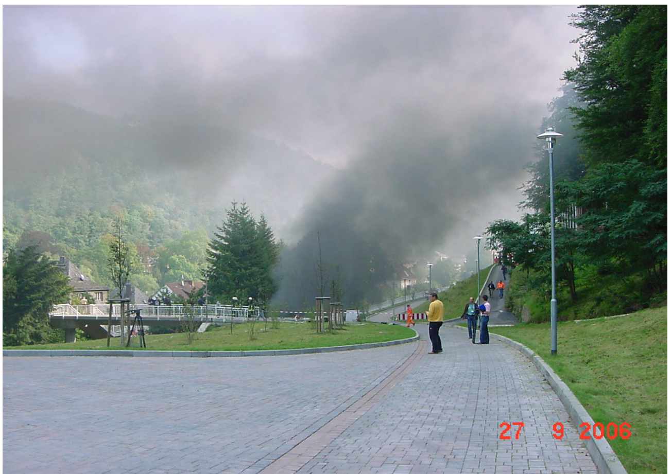
Picture 38: The smoke as discharged from exhaust station #06, influenced and re-directed by the west wind, viewed after 29 minutes from the west.
