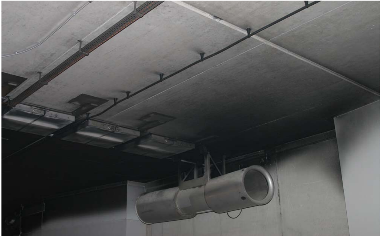
Picture 56: After the test, there was a blackened 1 m high strip to be seen on the northern wall next to the ceiling, extending over 100 m from the smoke extracting station #05 to the next one. During the fire alarm the jet fans in the western division operated in reverse mode without contact to the smoke. However, a small fraction of smoke circulated in the fan niche along the ceiling above the jet fan.
