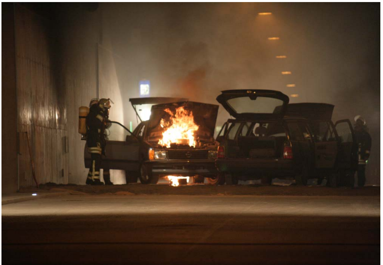
Picture 25: The developing of the fire in the engine compartment (the batteries have been removed in advance) with slight dimming of the ceiling lights, viewed after 4 minutes from the east.
