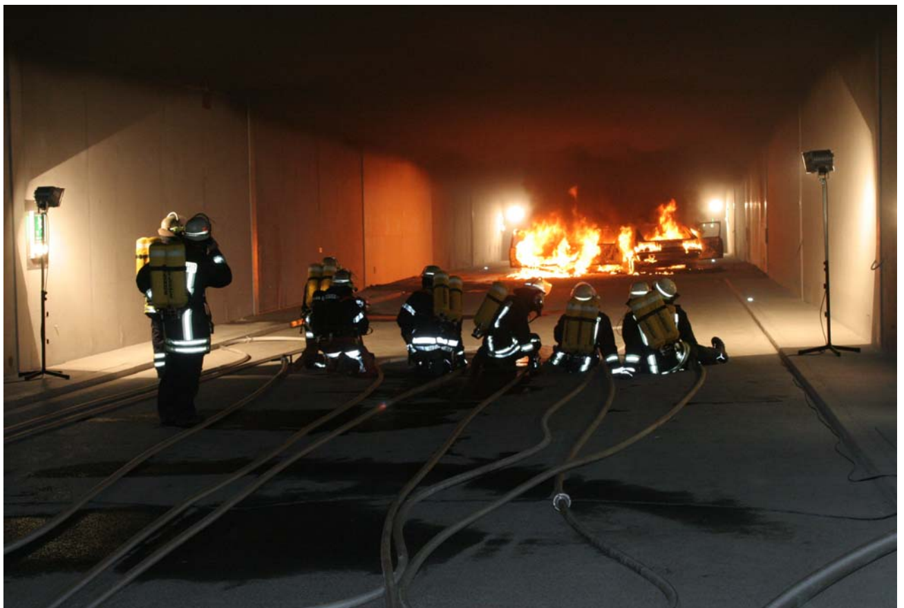
Picture 44: The cars were still burning, viewed after 27 minutes from the west, and still there was a stable smoke layer (stratification by density difference) when the fire brigade prepared itself for the attack.
