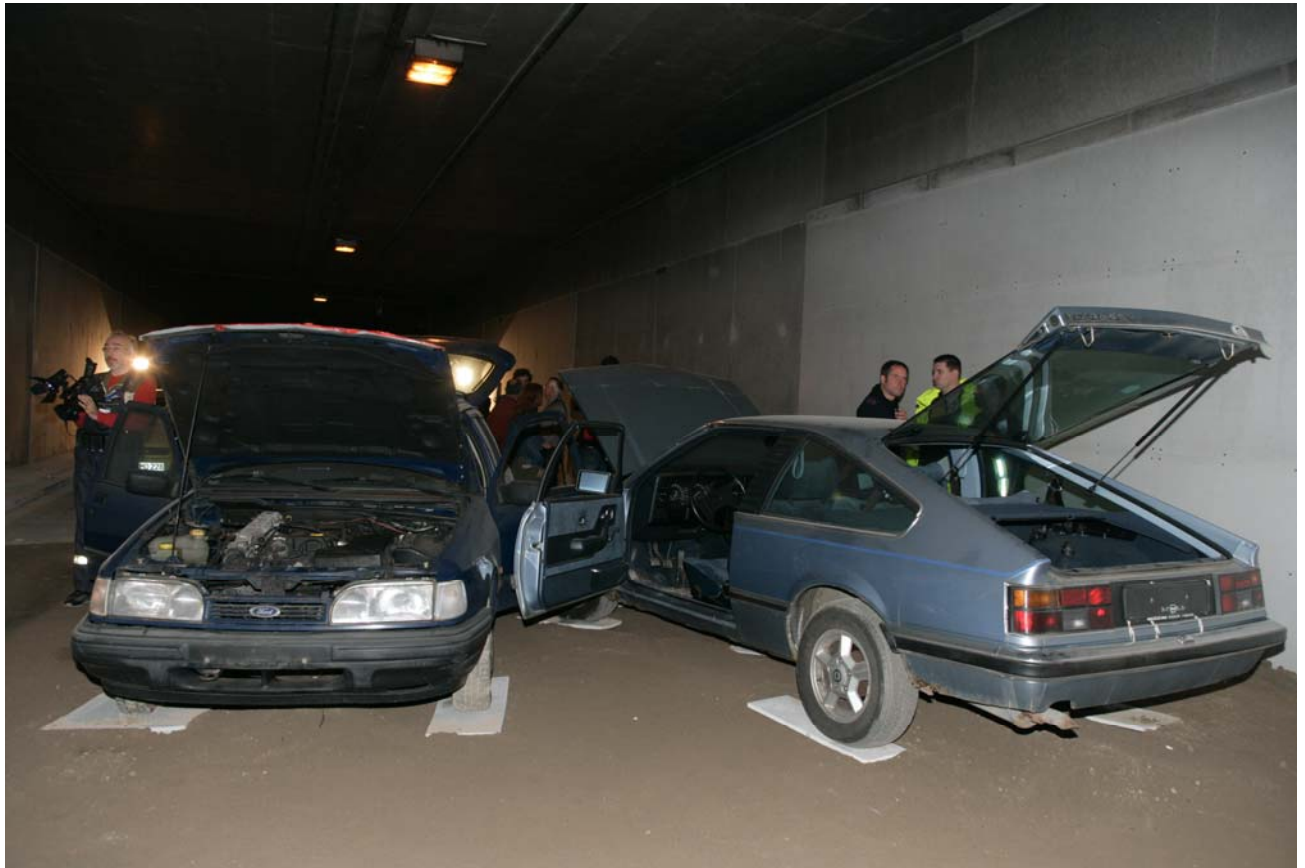
Picture 20: The Ford Sierra filled with 30 litres of diesel oil and the Opel Monza with 30 litres of petrol, each with 2 spare tires and all doors and hoods open, placed on 25 mm fire retardant plates.
