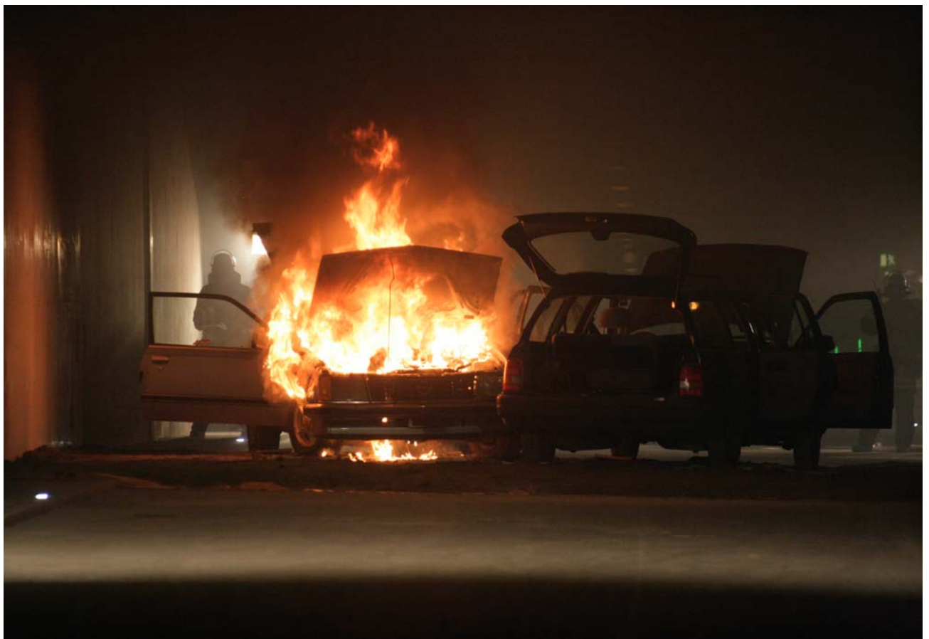
Picture 29: The fire viewed after 10 minutes, when the smoke layer was still stable and darkening the entire division of the tunnel between the two smoke extracting stations #05 and #06.
