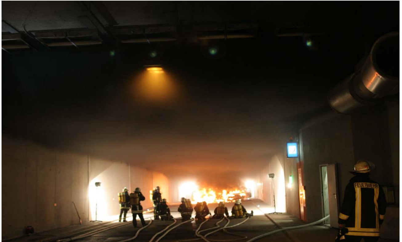
Picture 45: The cars were still burning, viewed after 28 minutes from the west, and still there was a stable smoke layer (stratification by density difference) when the fire brigade lifted up the water guns connected through a size B hose with the adjacent hydrant located in a separate chamber of the tunnel niche and served from a central pumping and pressurisation unit located in front of the control building.
