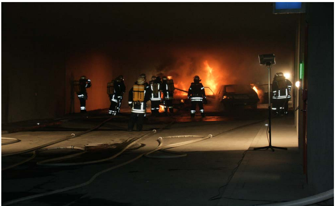
Picture 48: The attack from the west side started 28 minutes after ignition and ended 1 minute later. All over the testing and the extinguishing period the stratification of the smoke remained stable.
