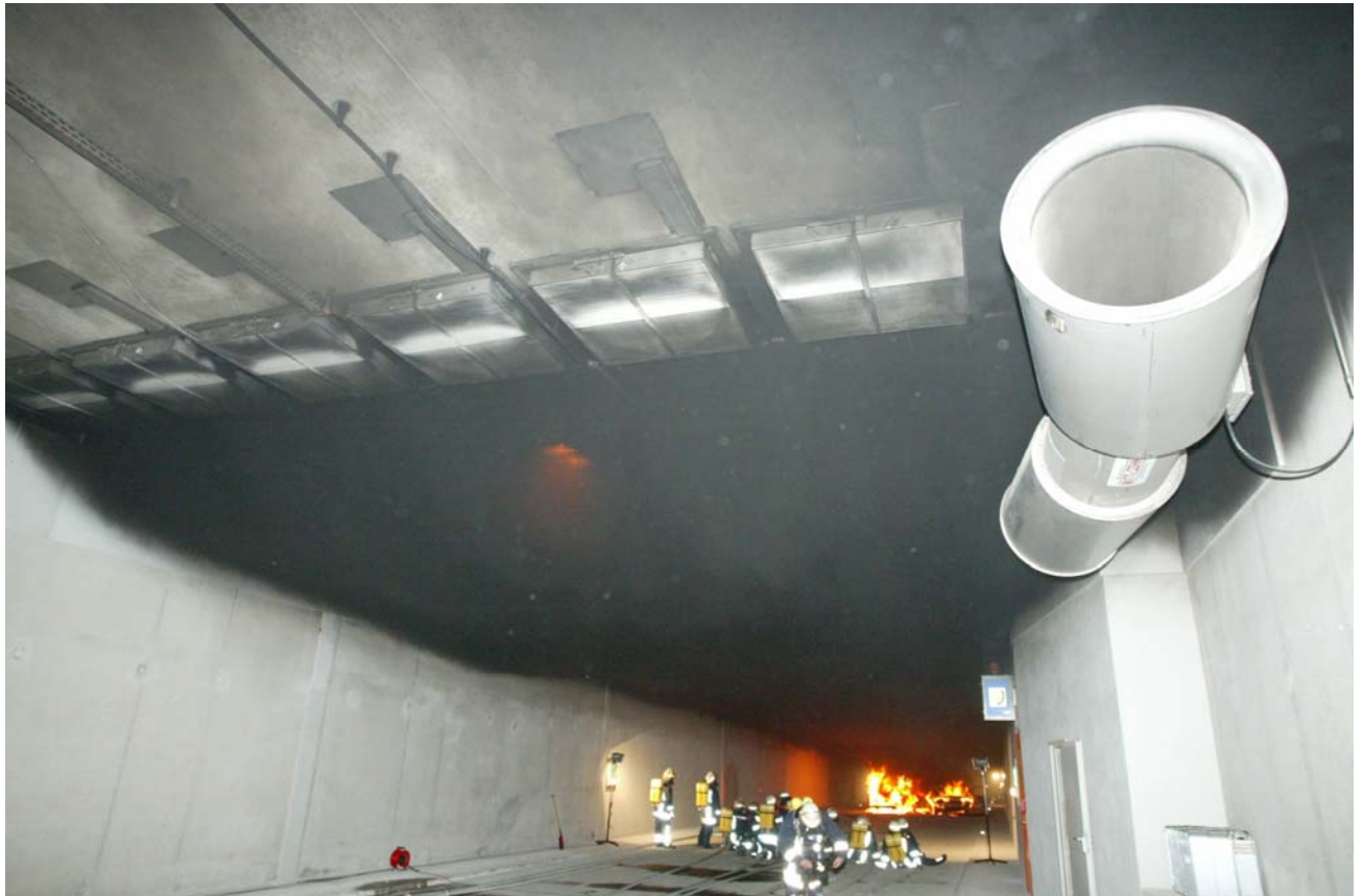
Picture 41: The stable flow of the smoke layer below the ceiling heading towards the extracting station #05, viewed after 23 minutes from the west, the smoke layer had a height of about 1 m which equalled the height of the heat protection on the walls. As the jet fans of the western division ran in reverse mode they had no contact with the smoke layer and no smoke could by-pass the extracting station #05.
