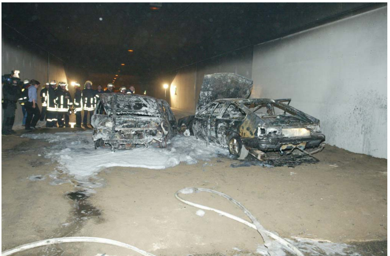
Picture 50: The wrecked cars, viewed after the fire has been extinguished by medium foam. The light fittings and glasses fixed to the ceiling were blackened from soot and the heat sensor cable, the radio antenna, the lighting cables, the loud speakers and some measuring apparatus have been damaged.
