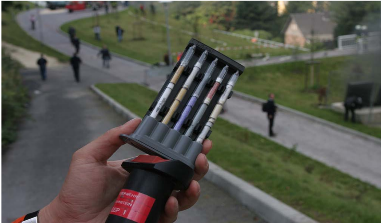
Picture 39: The simultaneous test set with hand pump and 5 Dräger tubes to measure several inorganic, burnable gases at once in order to control the distribution of noxious gases in the vicinity of the exhaust shafts and the next housings (the measured values were absolutely zero).
