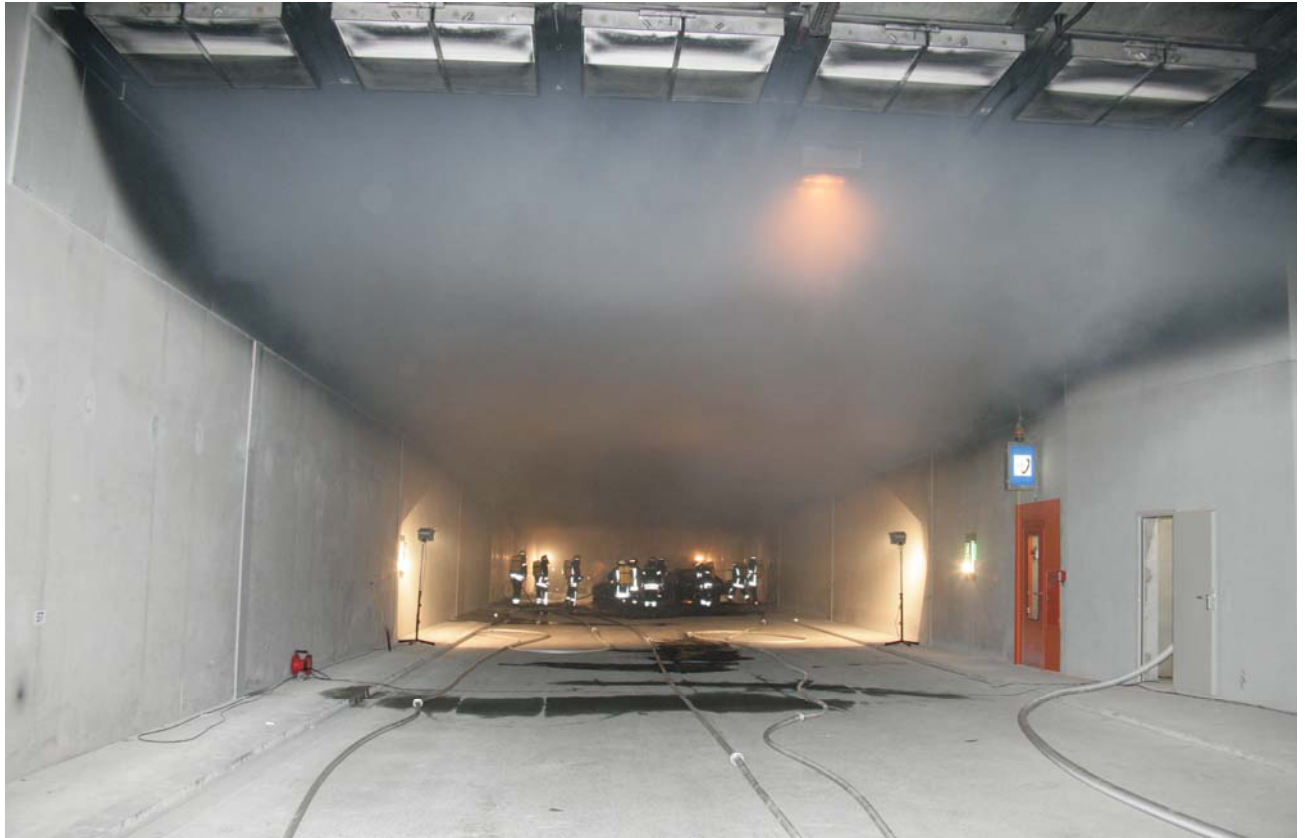
Picture 49: The steam layer replaced the smoke layer, viewed after 32 minutes from the west. The walls were blackened only along the ceiling on a 1 m high strip. The emergency phone booth and the emergency lightings remained visible and the hydrant niche remained accessible all the time.
