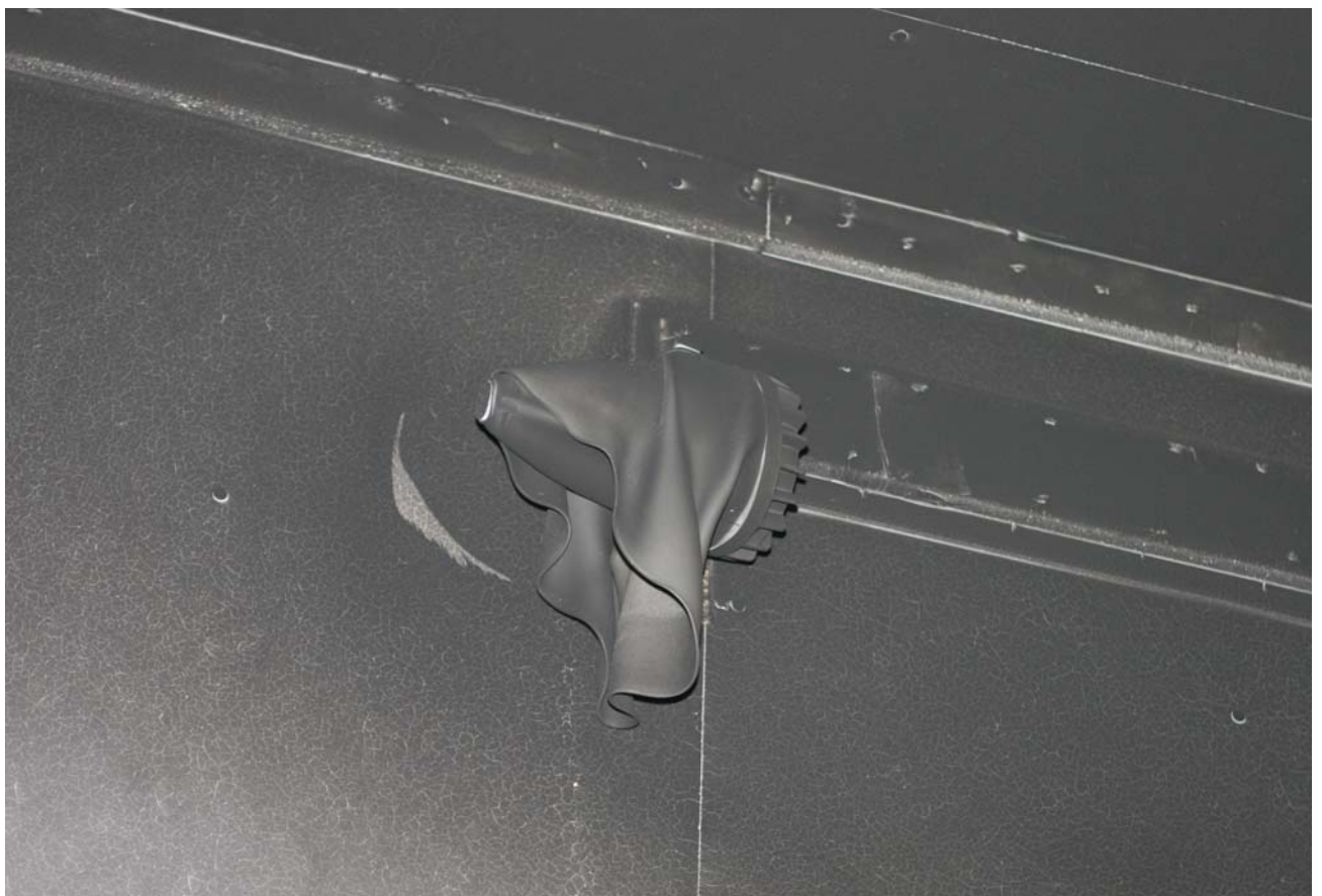
Picture 53: The loud speaker's shell was made of plastic and fixed to the wall near the ceiling where it rapidly melted in the hot smoke layer.
