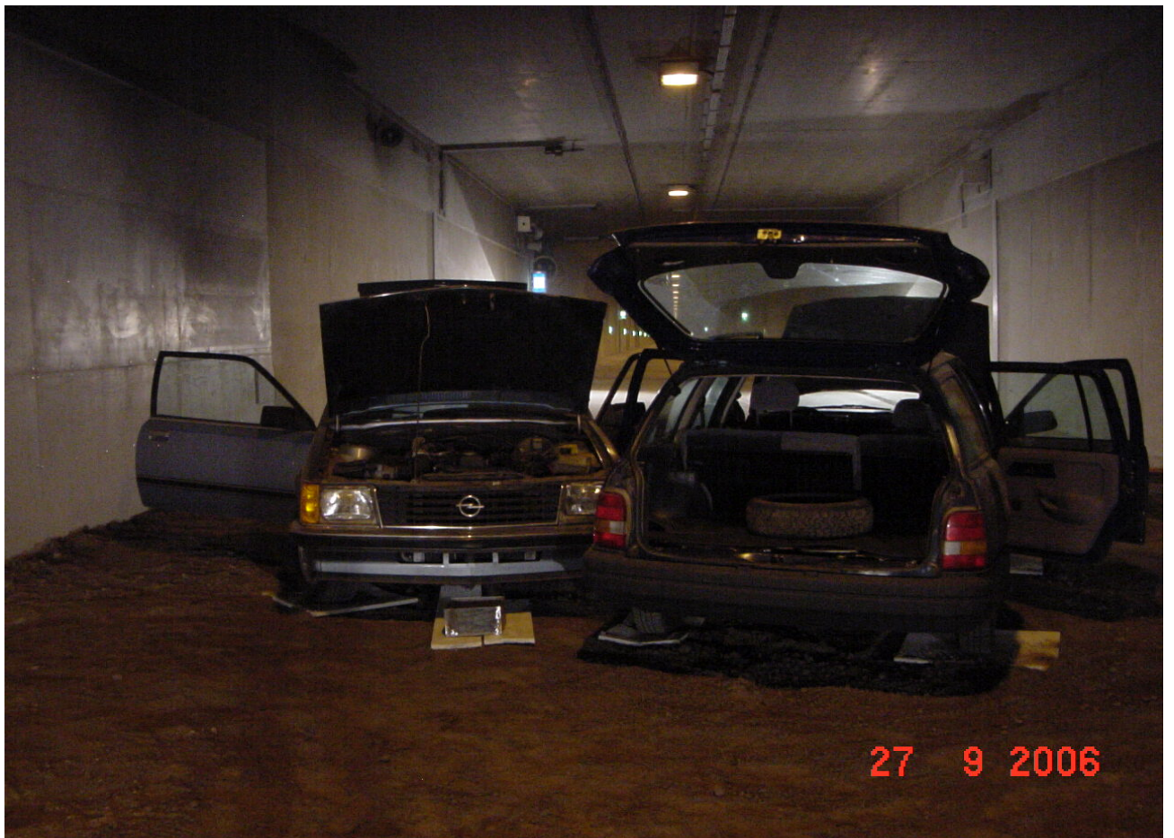
Picture 23: The placing of the ignition box (filled with 5 litres of petrol) under the gas-engine, the cars were set up in a 10 cm high sand bed (with wet cable sand), viewed from the east (the measuring apparatus have been installed under the ceiling in distances of 20 m to 30 m from the fire place).
