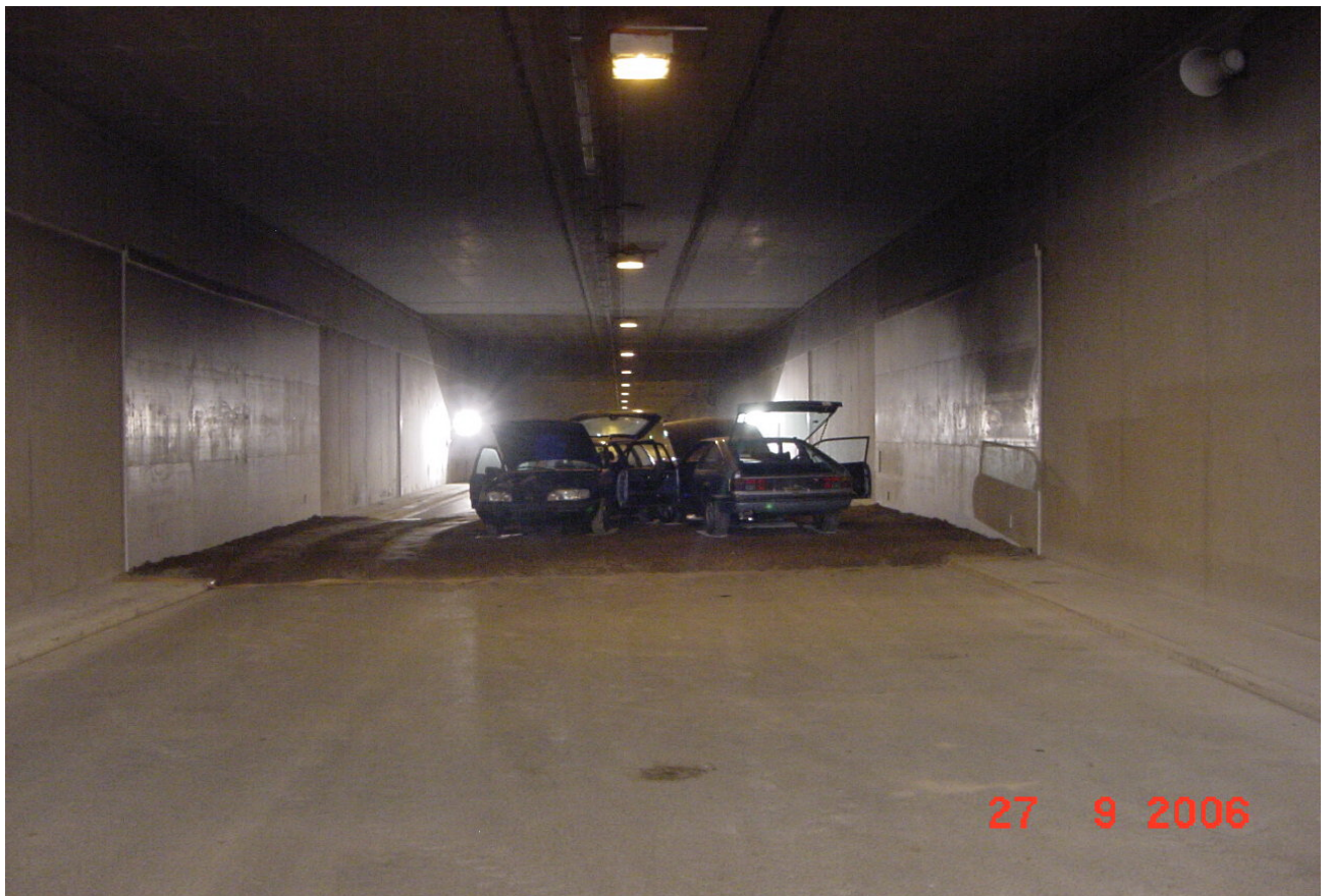
Picture 21: The arrangement of two passenger cars in the fire test bed, the walls were heat protected by covers of 25 mm fire retardant plates, 5 m high and 10 m long, as well as 1 m high and 100 m long.
