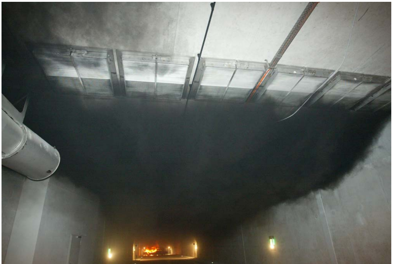
Picture 40: The stable flow pattern of the smoke layer below the ceiling heading towards the extracting station #06, viewed after 12 minutes from the east, all escape routes, emergency walkways and stair cases were kept free from smoke over the entire test period, but ceiling lights were darkened and cameras went blind so that no useful video image from near the fire place was available in the control room.
